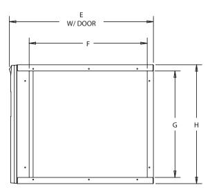
Inlet Side Return Duct Connection
